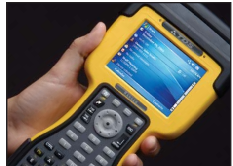
The Ranger's color display remains visible in direct sunlight, with powerful illumination for low-light conditions.
